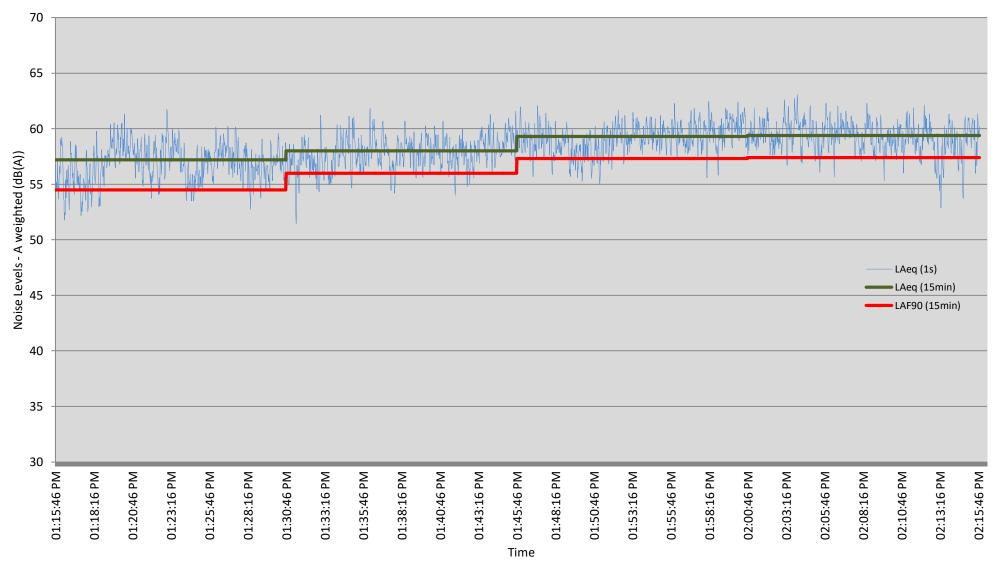
Pakiri Sand Extraction - Noise Level Measured at Position 1 - 13<sup>rd</sup> June 2019 Wind direction: North-West - Wind Speed: 1.5 m/s to 2.9 m/s - Swell: 0.8 m
