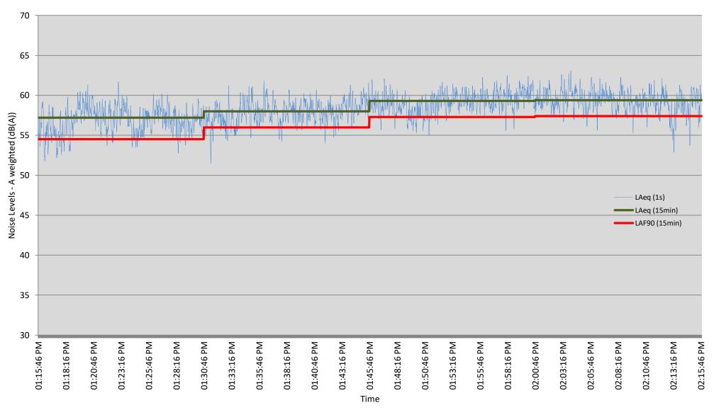
Pakiri Sand Extraction - Noise Level Measured at Position 2 - 13<sup>rd</sup> June 2019 Wind direction: North-West - Wind Speed: 1.5 m/s to 3 m/s - Swell: 0.8 m
